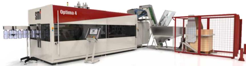
position. With 6 cavities version, it is possible to produce bottles up to 3L, with nominal working speed 7000 bph of 1l. suitable for bottle 200 ml–3000 ml. **Optima 4MAX** is 4 cavities machine with nominal working speed 7000 of 1L, suitable for bottles up to 6000 ml. **Optima** machines are designed for customers interested in high advanced and reliable blower.
